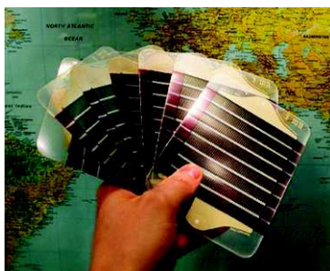
Fig. 1.2.1 Photovoltaics modules manufactured at DTU (Denmark Technical University) on PET substrate. The modules are made of 8 cells on series.
