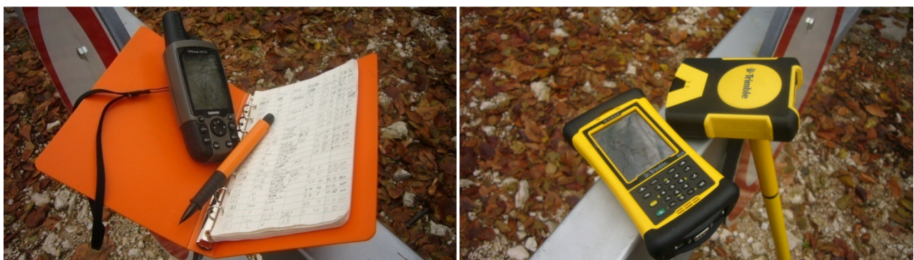
Figure 12 - Consumer-grade receivers with mapping GIS functionality (left) professional receivers for mapping GIS survey with post-processing correction (right)
