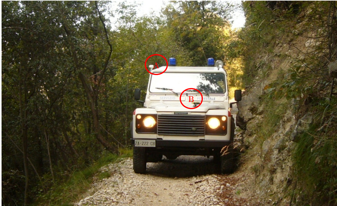
Figure 13 - Application of an external antenna for Consumer-grade GPS receivers with differential correction (A) and external antenna with Bluetooth connection for Mapping-grade GPS receiver (B)
