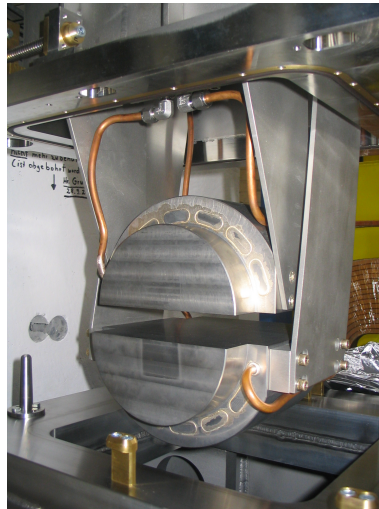
Figure 2.7: Photograph of one of the target slits to cut the acceptance in the vertical (Y) direction.
