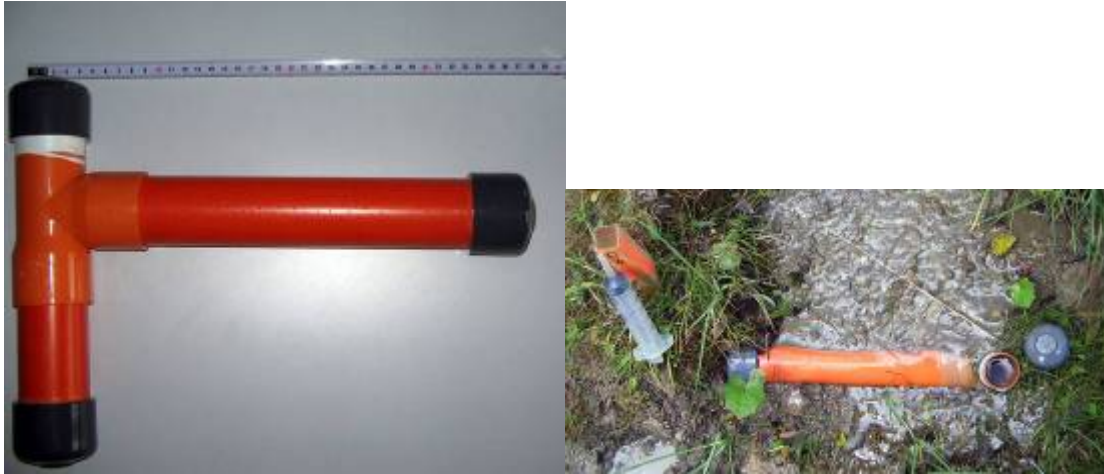
Figure 12: Overland Flow Detector after construction (left) and in place in the field; the cap was removed to show the device filled with surface runoff after a storm event.
