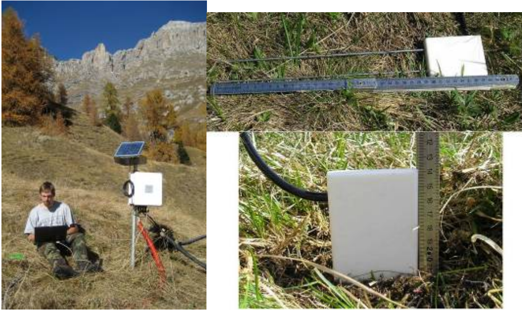
Figure 14: water content reflectometer (left); probe and stainless steel rods (right).
