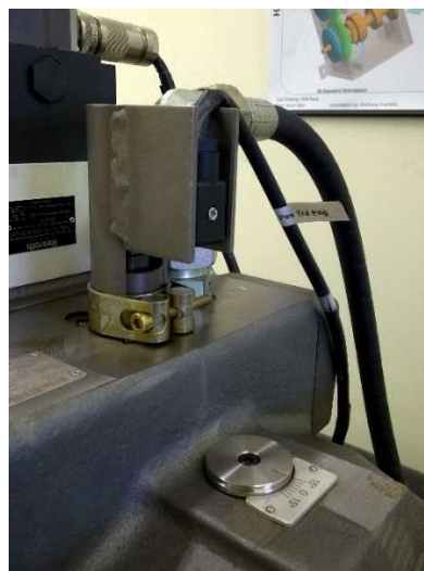
Figure 6.15: A view of the mechanical displacement feedback of the Engine Simulator.
