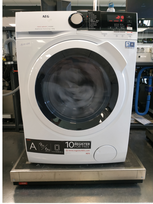
Figure 5.3: The Experimental apparatus. WD machine on balance.
