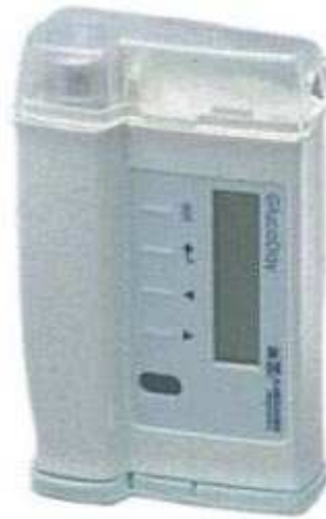
Figure 1.7: The Menarini GlucoDay ® device [63].
