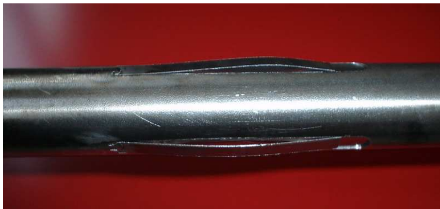
Figure 6.6: Detail of the steel tabs built up to guarantee the electric contact between the stainless steel tube and the Niobium target.
