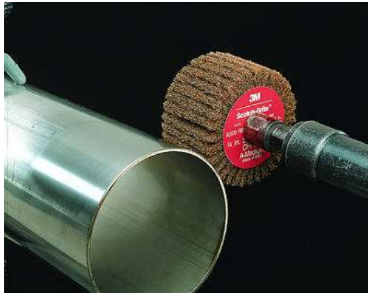
Figure 3.3: Scotch Brite TM tool used for mechanical grinding inside monocell cavities
