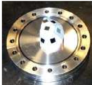
Figure 7.1: Sampleholder for 10x10 mm quartz substrates. It allows changing the deposition angle systematically.
