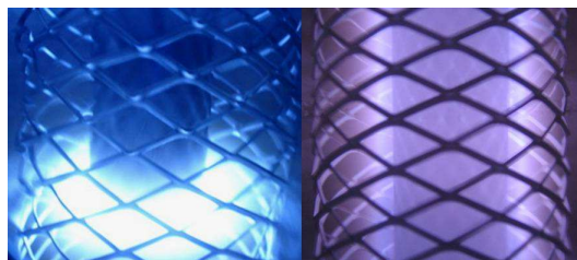
Figure 8.8: Pictures of the plasma discharge in the bias magnetron configuration. On the left the plasma is confined by an internal magnet. On the right the plasma is spread along the cathode due to the magnetic field of two external coils as in figure 7.19.
