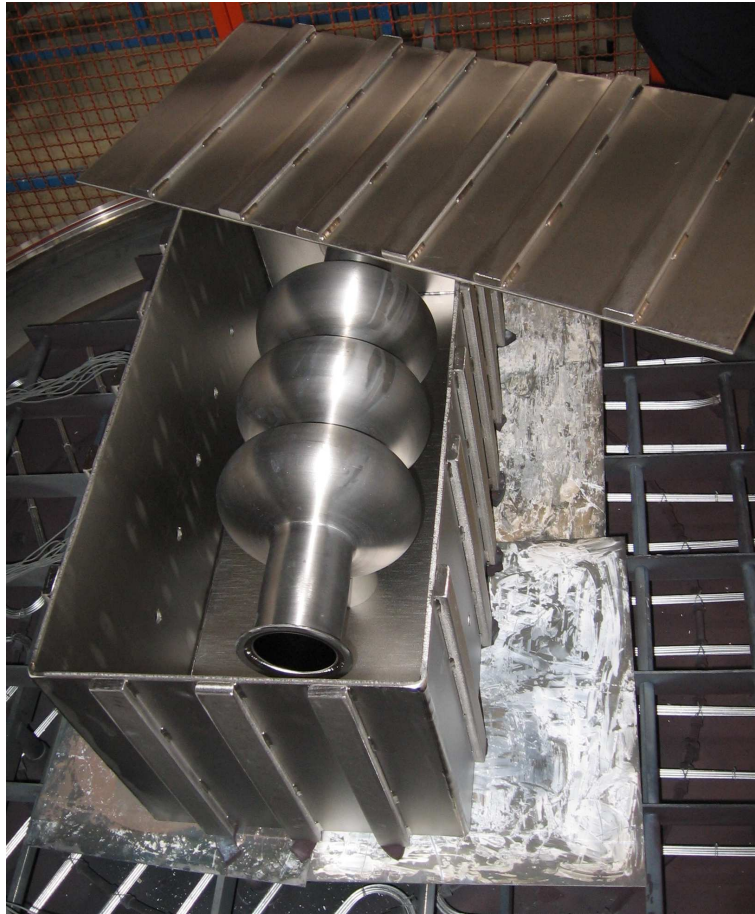
Figure 3.18: The 3-cell niobium cavity in the titanium box, waiting for the high temperature baking.
