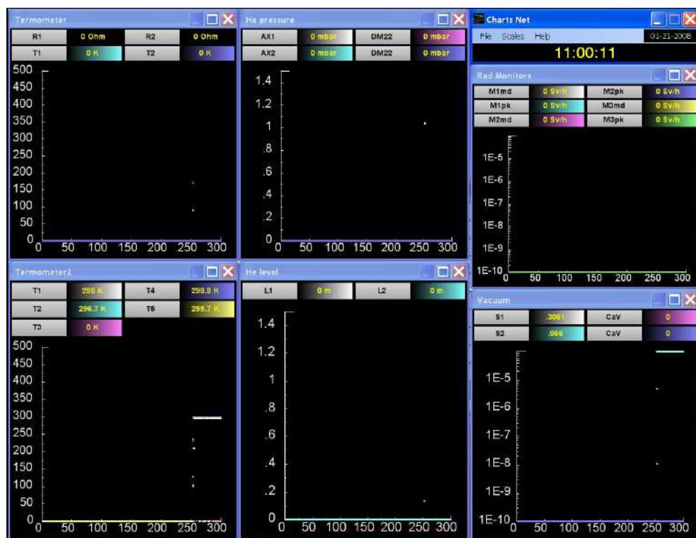
Figure 5.15: Screen shot of the monitoring real time visualization of data software CHARTS, developed in Visual Basic ..... in order to draw all monitored data collected by the software GUARD.
