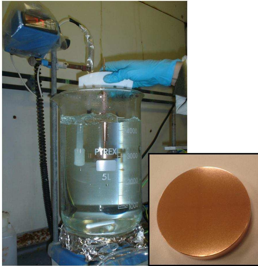
Figure 3.15: During SUBU the solution should be energetically stirred in order to avoid the formation of a viscous layer that reduce and finally blocks the etching. The surface finishing after EP, SUBU and passivation is visible on the plate down to the right.
