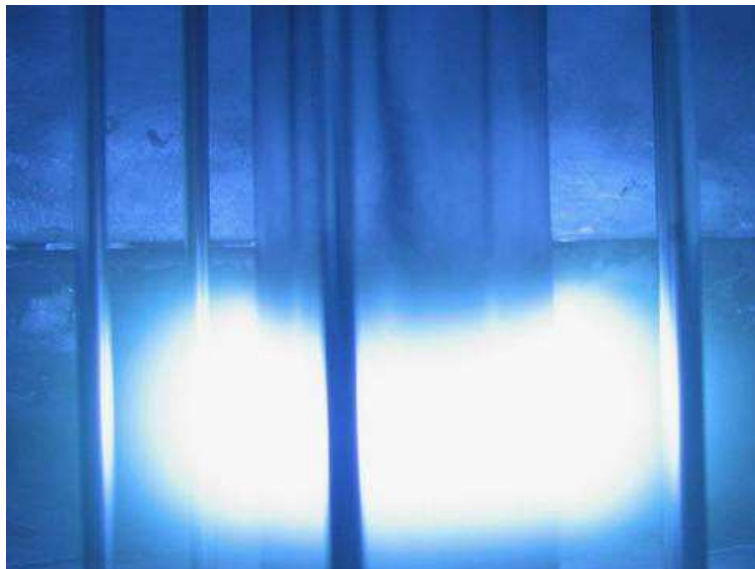
Figure 8.10: Pictures of the plasma discharge in the bias magnetron configuration. The plasma is confined by an internal magnet leveled with the cavity cell.
