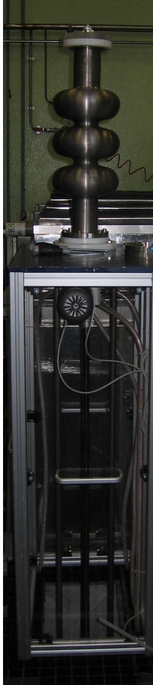
Figure 3.22: Picture of the 3-cell spun niobium cavity monted on the HPWR system.
