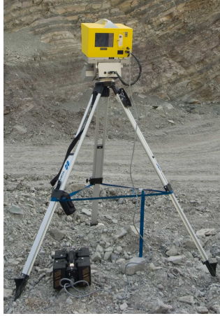
Figure 2.5: Optech ILRIS 3D TLS. The knowledge of the minimum acceptable distance of acquisition is necessary both for planning scan acquisition and for a valid intensity evaluation and interpretation. This information must either be asked to the manufacturer or obtained via preliminary tests on calibrated targets.
