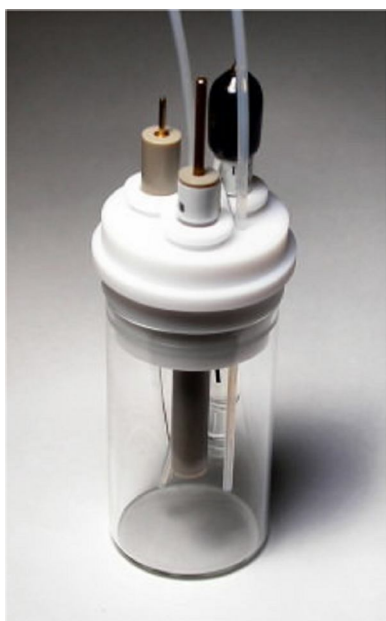
Figure 7.1 Typical oxygen-free pyrex glass cell used in the electroanalytical measurements. http://www.xenosystem.com/ckseo/als/010914-2.jpg
