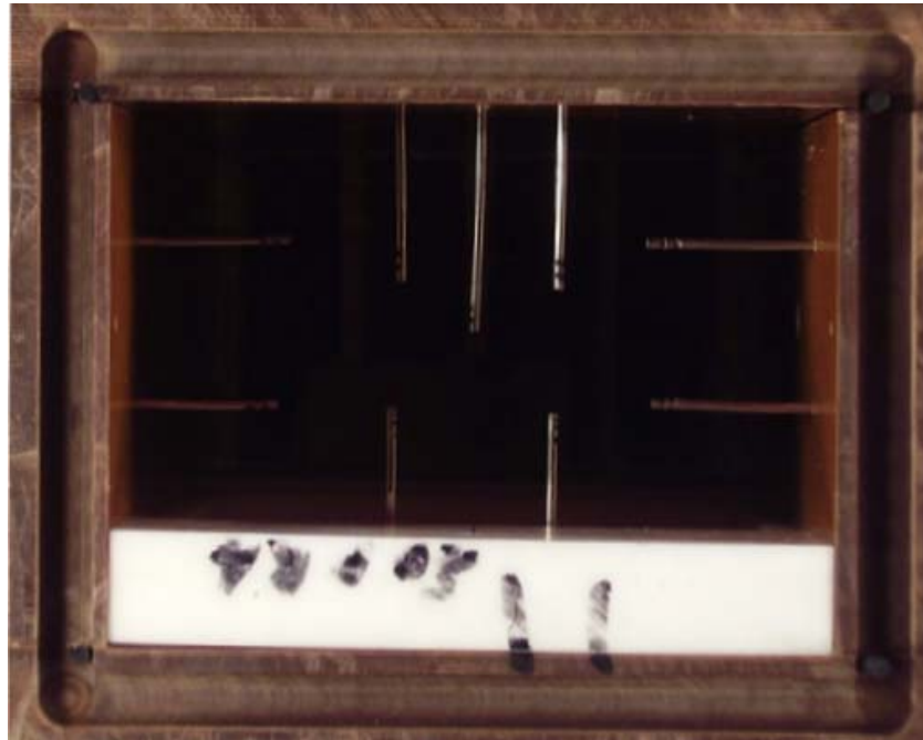
Figure 135. Photo of the thermocouples distribution at the inlet of the test section.
