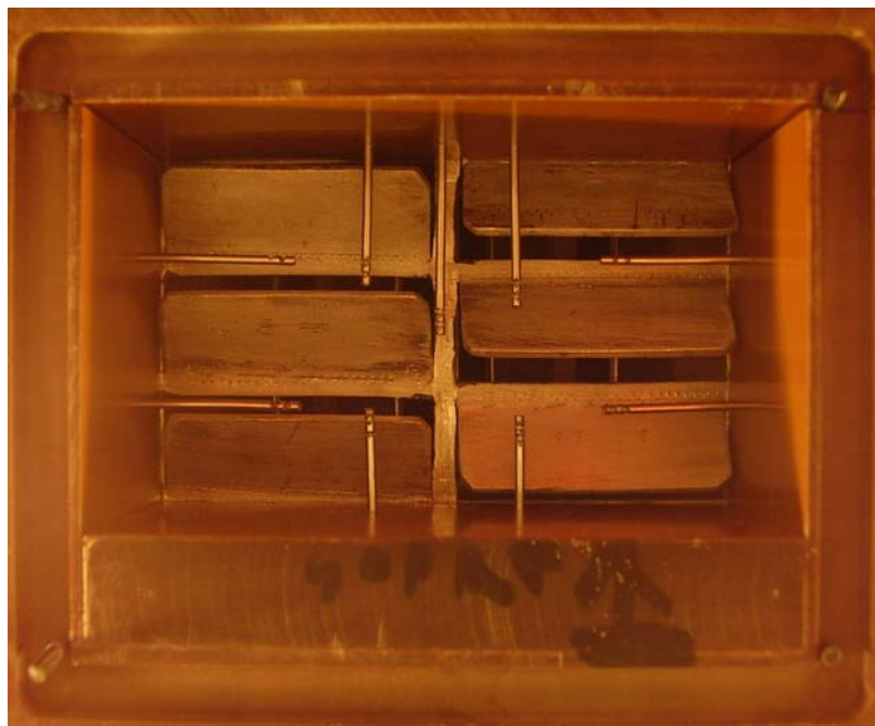
Figure 137. Photo of the thermocouples distribution at the outlet of the test section.
