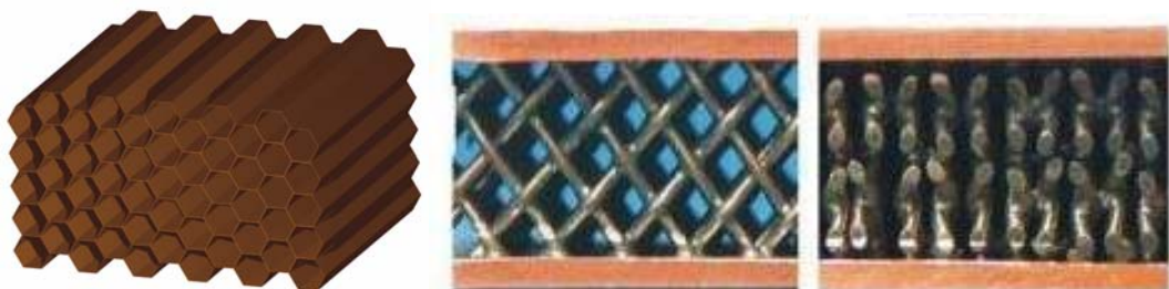
Figure 79. Example of copper honeycomb (left) and 2D copper structure (right) (photo by Tian et al. [19]).
