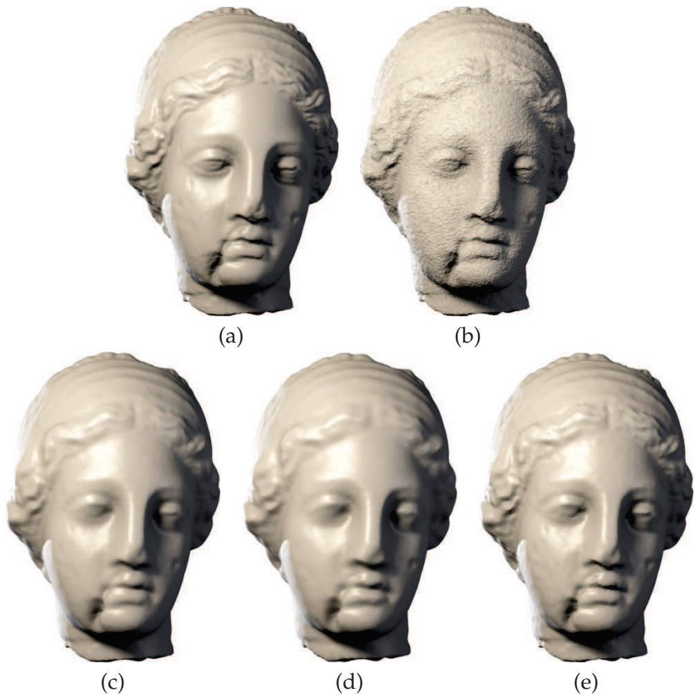
Figure 2.6: igea mesh: (a) Noise-free mesh; (b) noisy mesh; (c), (d) and (e) the MCF, BLF and SDF-NL restoration respectively.
