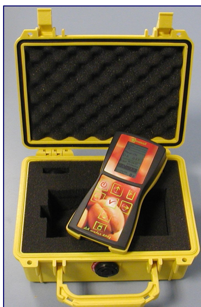
Fig. 3.1. Portable spectrometer developed in the laboratory of Prof. Guglielmo Costa. Vis spectroscopy was used to develop an index characterizing ripening changes in peach fruit.
