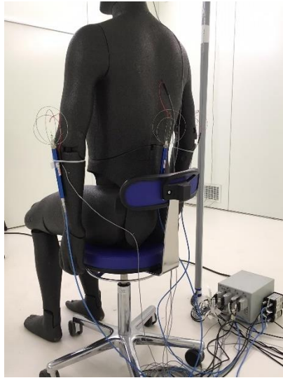
Figure 5.26 - Position of the anemometers for air velocity measurements.
