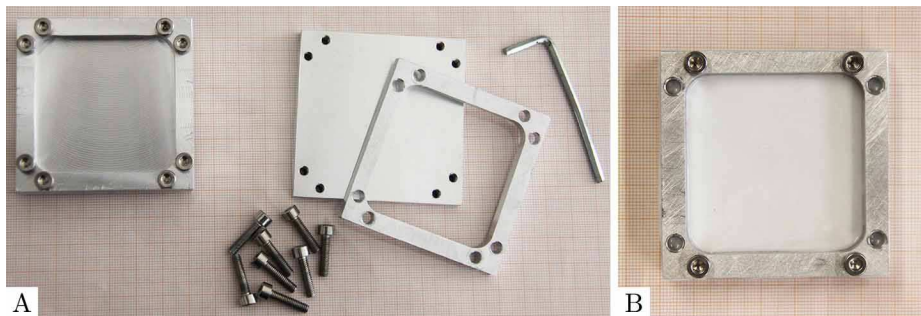
Figure 2.8 Aluminum frame used to assemble HM. The frame comprises a lower component to support pericardium and an upper element to border liquid polyurethane (A). DBP was fastened to the frame before polymer was poured (B).
