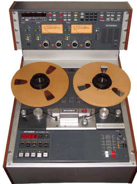
Figure 2.11: A Studer A810 (VUK version) tape recorder [36]. In VUK versions, a separate console – not modeled by our app – houses the VU-meters, the channel control commands, and the monitor speaker.
