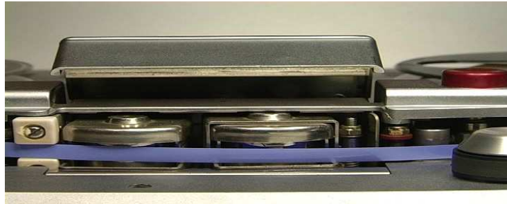
Figure A.1: A frame of the class End of Tape : the capstan is detached from the tape.
