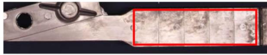
Figure 3.4. Position of specimen for radiographic testing in the stepped wedge of the casting.
