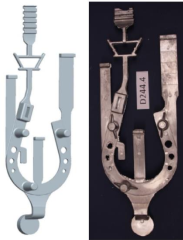
Figure 3.2. Horseshoe-shaped casting designed to exacerbate the generation of defects.
