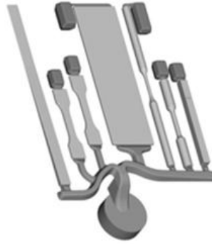
Figure 5.6. Reference casting designed to minimize the generation of defects.
