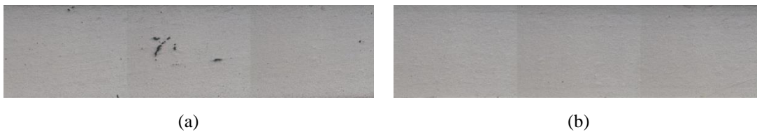
Figure 4.15. Optical micrographs of the zone near the fracture surface of: (a) a scrap casting ( a_{RMS} = 13.73 \text{ m/s}^2 ) and (b) a sound casting ( a_{RMS} = 62.24 \text{ m/s}^2 ).
