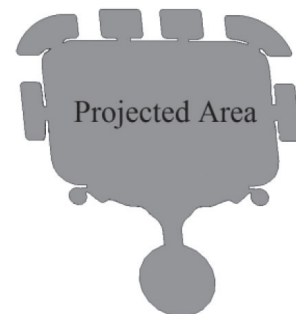
Figure 18. Projected area of the die in the parting surface.
