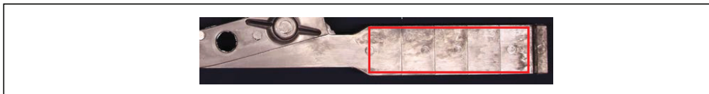
Figure 1: Position of specimen for radiographic testing in the stepped wedge of the casting
