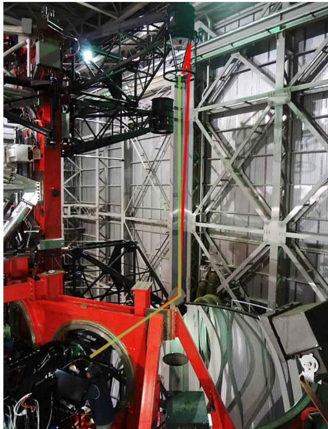
Figure 6-4: The Pathfinder at the telescope. The green beam is the beam used in configuration #1 for the materialization of the bearing rotation axis, while the red beam was used in configuration #2 for the materialization of the telescope optical axis.
