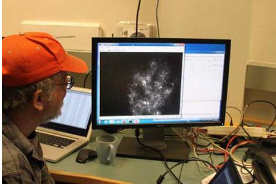
Figure 6-21: Pathfinder first light on the AVT camera. The image was very aberrated and out of focus, but enough to reach the first Pathfinder nighttime goal, the mere acquisition of an on-axis star.
