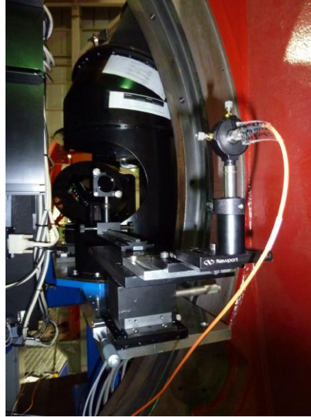
Figure 6-13: The AL mounted on the additional breadboard. The IRTC is also visible.
