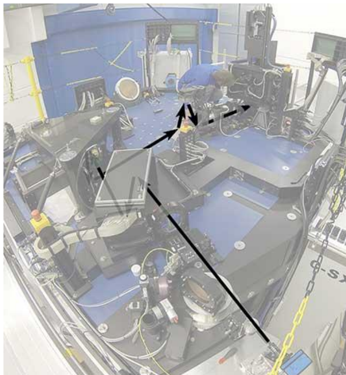
Figure 7-11: Light from the telescope enters at lower right and passes through the collimating lenses before bouncing off a flat mirror. The second reflection takes place at the surface of a 349 actuator deformable mirror before continuing on to the midline of the instrument. Reflections off the piston mirror and a visible-infrared dichroic send the radiation to the FP20 lens system at upper right. The K-mirror precedes a final mirror, which sends the light upward into the wavefront sensor.
