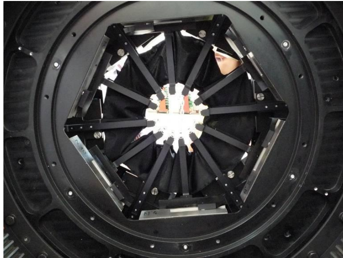
Figure 4-23: the elastic cloth that will mask the background light not passing through the SEs, preventing pupils' contamination.
