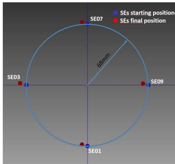
Figure 7-25: position of the SEs used for tip-tilt and focusing alignment of the AM, as seen from in front of the GWS entrance. The SEs were initially positioned on a cross pattern (blue circles) on a circle 68mm in radius, centered on the nominal center of the GWS focal plane. The pupils we got in these positions were highly defocused, so we moved the AM in focus, tracking the beam at the same time with the SEs. The red circles represent the positions of the SEs where we had, at a visual inspection, pupils with no defocus signal. The final positions of the SEs are shifted, on average, of 6mm in X axis and 2mm in Y axis wrt the starting position
