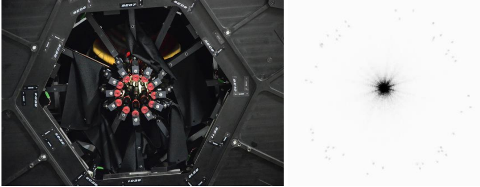
Figure 5-26: On the left, all the SEs illuminated by the collimated beam for a first rough tip-tilt alignment. On the right the small spots produced by the 12 SEs on the test CCD before the alignment. After the alignment, all the small spots will be distributed in 4 very small clouds (of few pixels). The central bright spot, whose centroid is our reference for the tip-tilt alignment, is produced by the collimated light not passing through any SE and focused by the PR-I on the center of the CCD.
