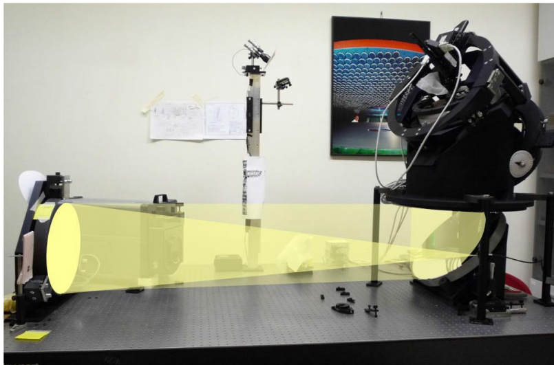
Figure 5-13: The optical setup used to align the PR-I, shown as Zemax layout (top) and in the lab (bottom).
