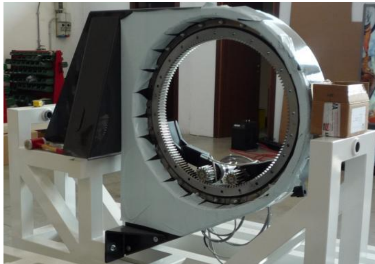
Figure 4-24: The bearing allowing the rotation of the GWS.
