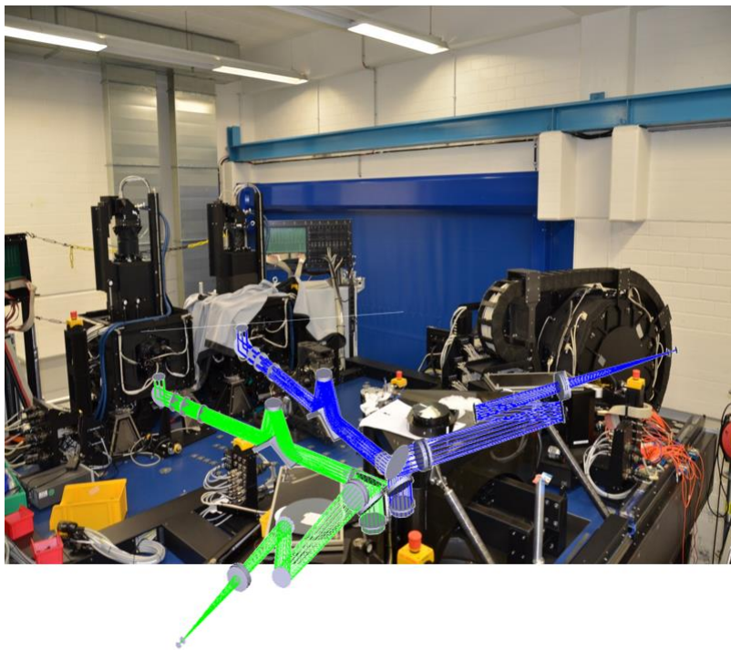
Figure 4-26: the light path inside the LINC-NIRVANA bench.
