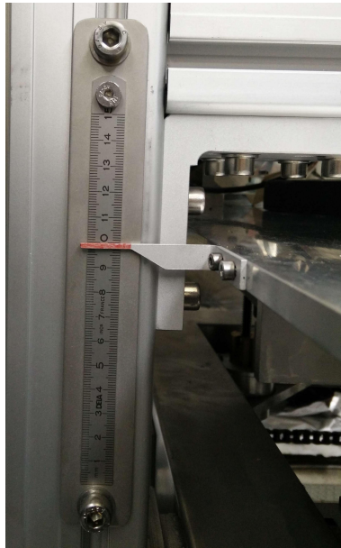
Figure 5.9: Measure installed on the side of the scanning table platform to read its height.
