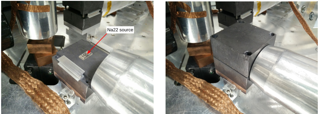
Figure 5.11: ^{22}\text{Na} source inside a detector collimator; with the collimator open (left) and closed (right). This setup is used for detector position calibration (Section 5.3.5) and external trigger gate calibration (Section 5.4.2). The collimator aperture is equal to the thickness of the ^{22}\text{Na} source which measures \sim 1.9 mm.
