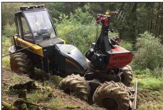
Figure 1.12: Anchor based winch-assist systems. From the top left: EMS Tractionline; Remote Operated Bulldozer; FFE winch-assist; Summit; T-Mar LC150; Ecoforst T-Winch; Herzog MW500; Haas three-point-winch
