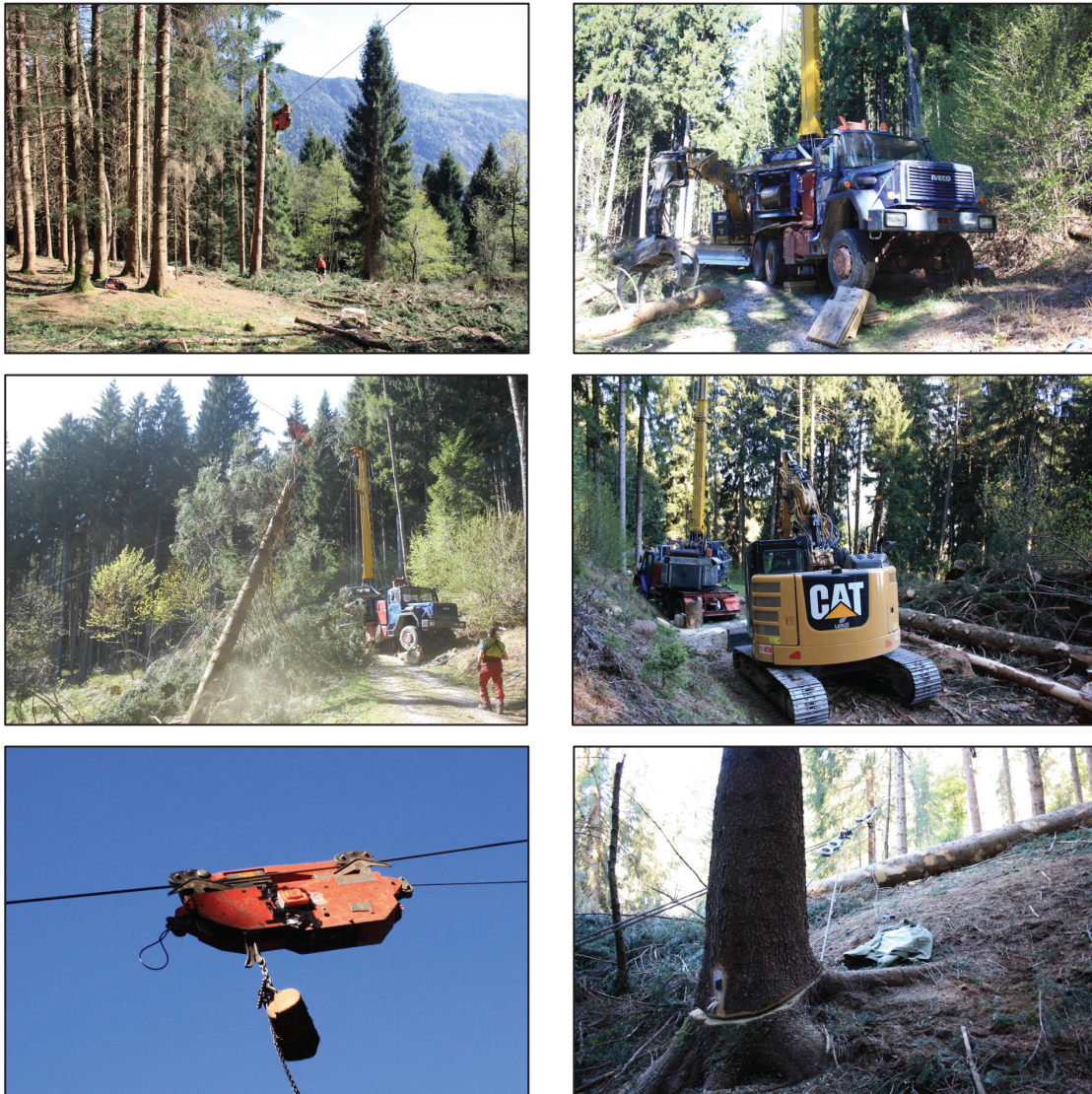
Figure 6.2: Photos of Site B. From the top left: Loading area; Cable yarder; Unloading; Landing; Carriage; Multiple anchor
