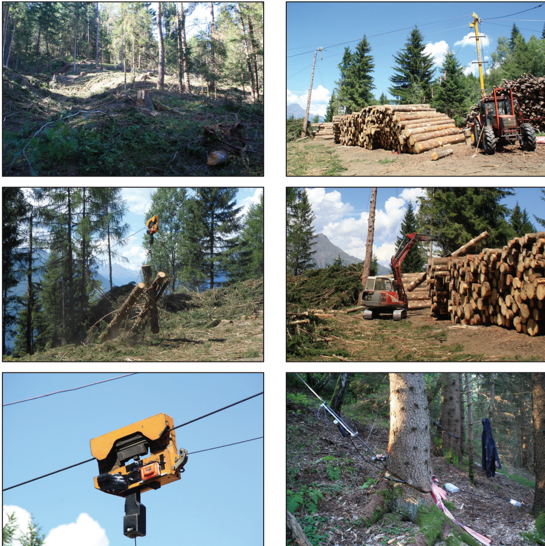
Figure 6.10: Photos of Site L. From the top left: Loading area; Landing; Inhaul; Excavator-based grapple loader; Carriage; Anchor
