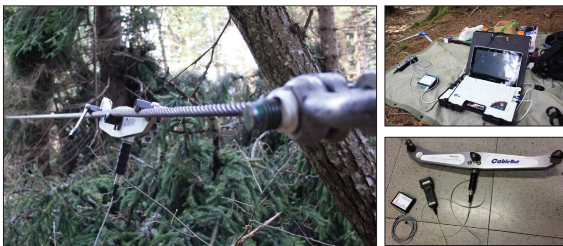
Figure 2.1: CableBull SR22/800XR tensiometer and recording set-up
