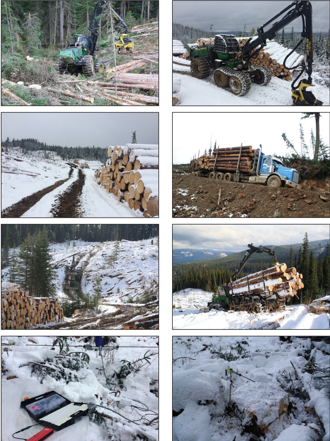
Figure 6.13: Photos of Site N. From the top left: Winch-assist harvesting operations; Harvester; Landing; Log-Truck; Winch-assist forwarding; Forwarder; Cable tensile force monitoring system; Anchor
