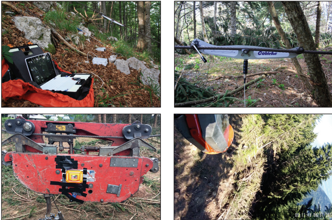
Figure 2.7: Sensors and tools mounted on a cable line. From the top left: cable tensile force monitoring system mounted on the skyline; CableBull tensiometer; Machine control unit mounted on a carriage; View of the Drift camera from the carriage
