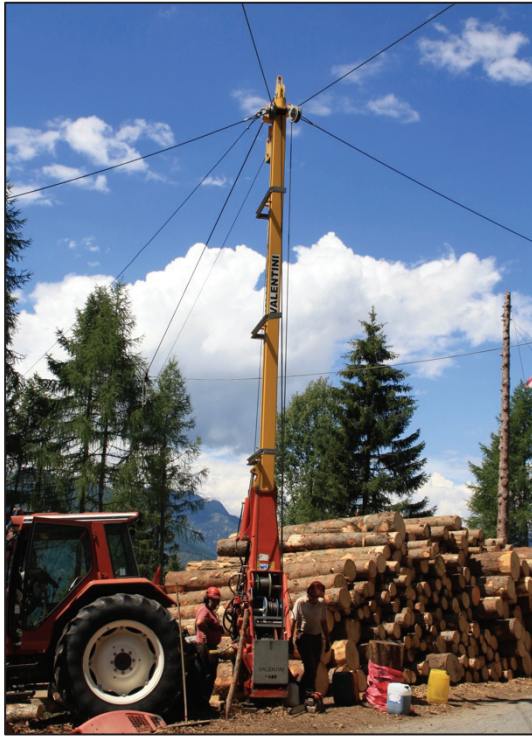
Figure 1.6: Tractor-based tower yarders
