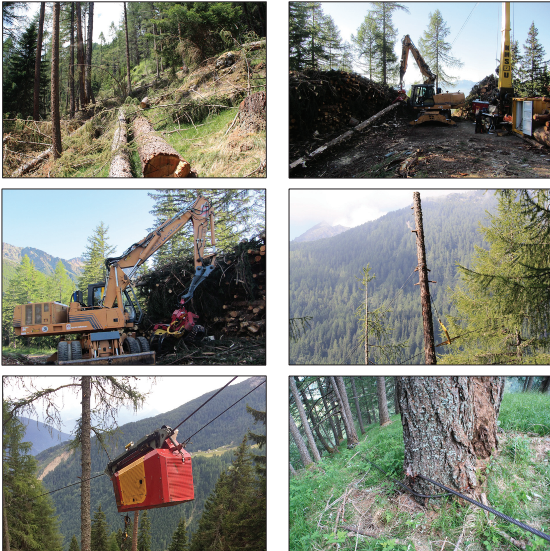
Figure 6.8: Photos of Site H. From the top left: Loading area; Landing; Excavator-based processor; Intermediate support; Motorized carriage; In-line double anchor
