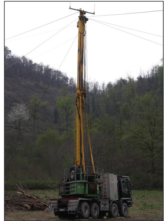
Figure 1.9: Truck-based and Processor tower yarders
