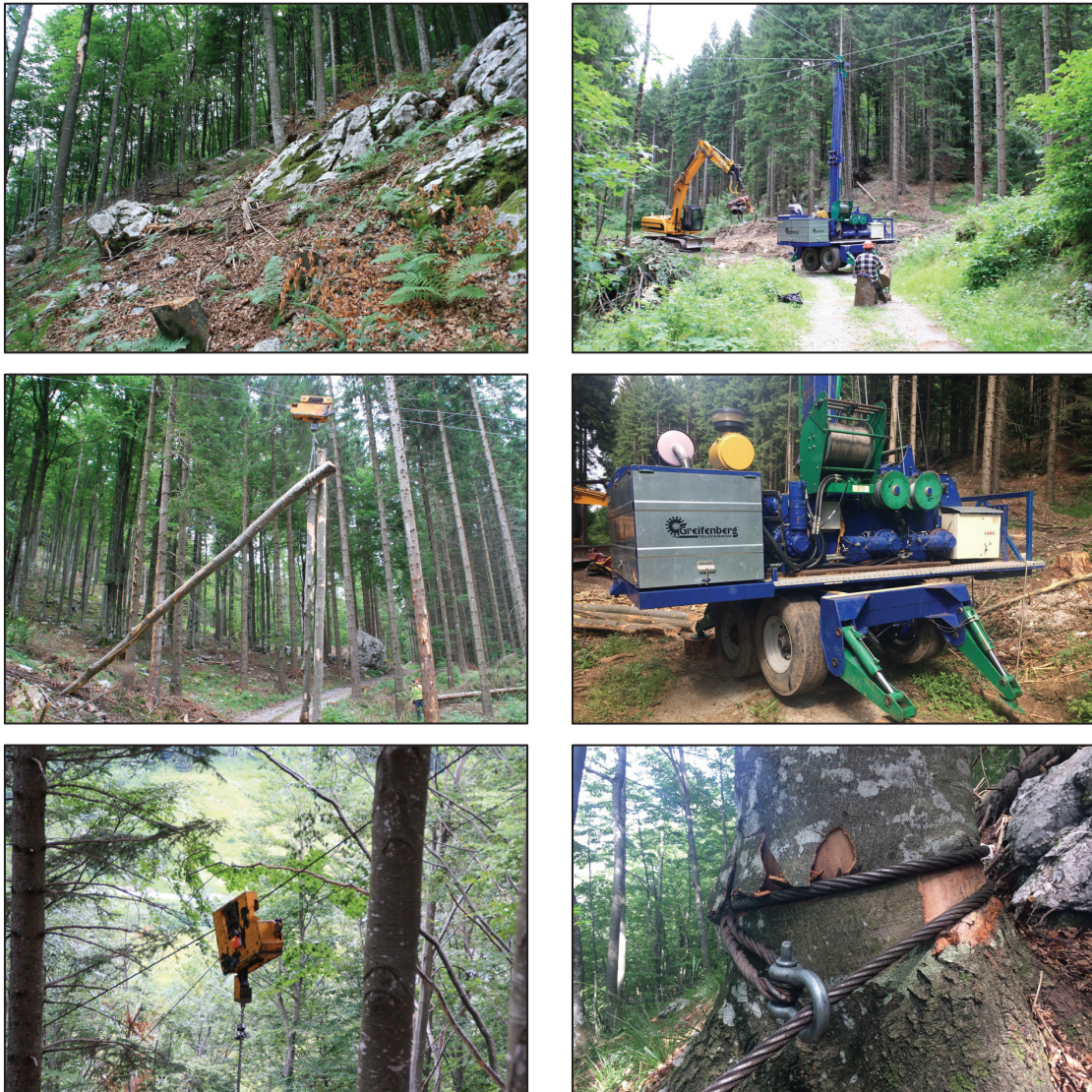
Figure 6.5: Photos of Site E. From the top left: Upper section of the Loading area; Landing; Unloading; Cable yarder; Carriage; Anchor
