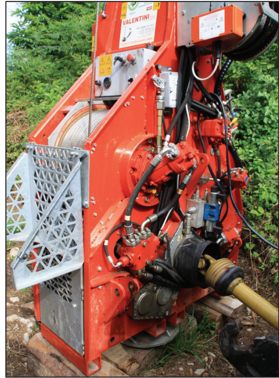
Figure 1.6: Tractor-based tower yarders
