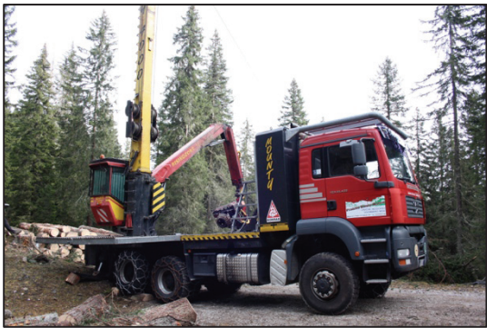
Figure 1.9: Truck-based and Processor tower yarders
