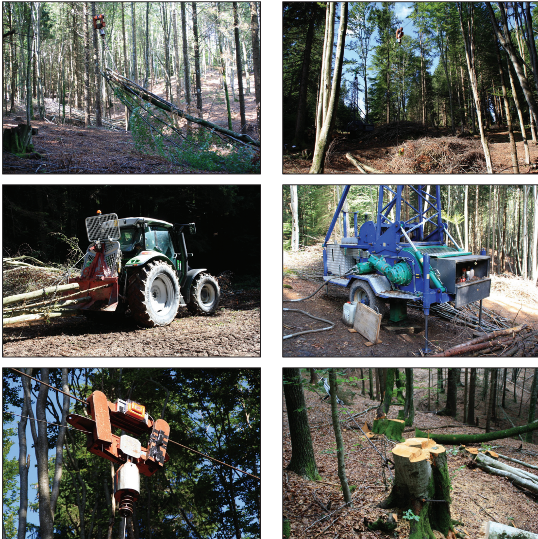
Figure 6.7: Photos of Site G. From the top left: Inhaul; Unloading; Tractor and winch used for cleaning the landing; Cable yarder; Carriage; Anchor
