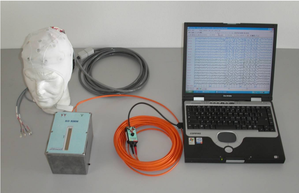
Figure 1.4. EEG-fMRI co-registration equipment.
