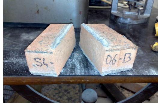
(b) Failure of a brick
