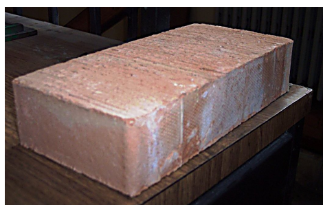
Figure 5.7: Solid clay brick used
