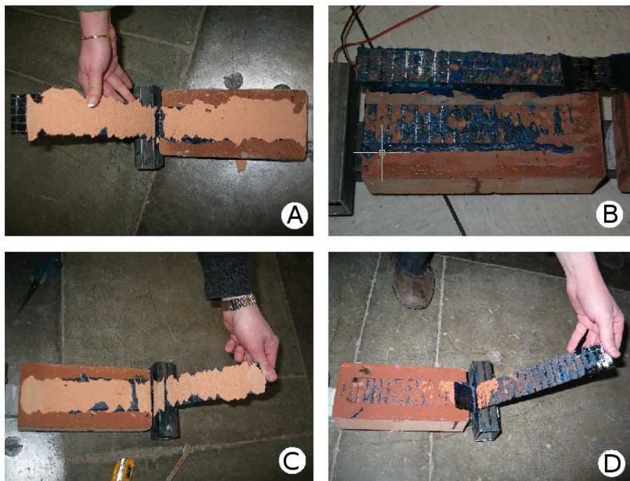
Figure 6.15: Typical failures: facing bricks S2 (A) and S4 (C), extruded bricks S3 (B) and S5 (D)
