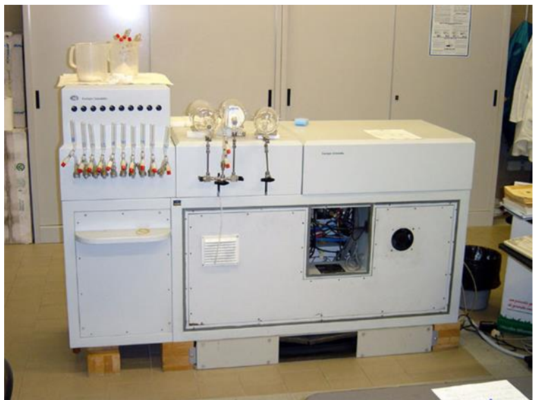
Figure 5.3.2 – Mass spectrometry of the Europa Scientific values (in the range, 2,5-2,7A) were reached at a slower rate (0,2mA/s)(Cavazzini, 2005).
