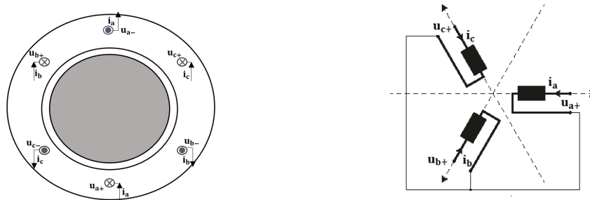
(a) Physical disposition of the coils (b) Star connection of the 3-phase windings.
