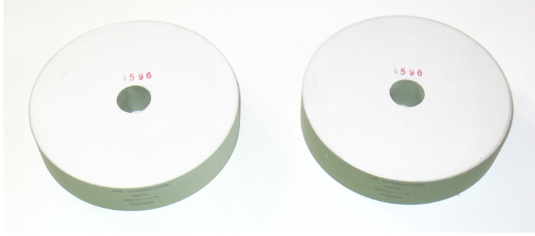
Figure 3.7: Disk resistors used for the damper
