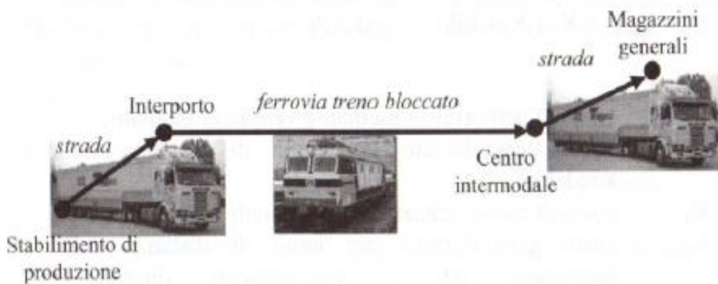
Figure 4.6. Example of complex pluri-modal cycle (source: Russo, 2005)
