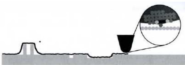
Figure II.5 Resolution limits in a conventional STM instrument. Images of step walls and holes are distorted when their size is comparable to that of the tip apex
