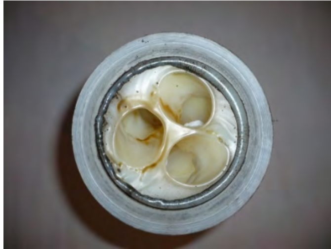
Figure 3.29: 3 ports helical grain after burning.
