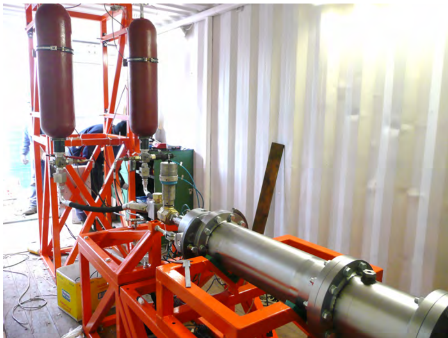
Figure 3.7: Full scale test bench during assembly.
