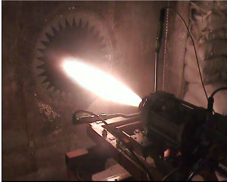
Figure 3.32: Wax test # 4 during burning phase.
