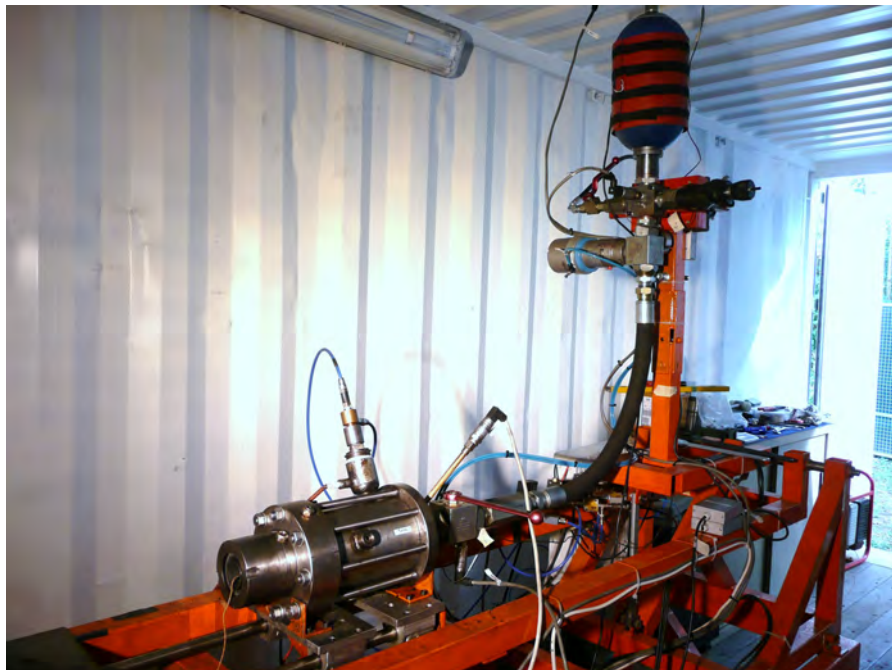
Figure 3.4: Small scale test bench installed on the fixed basic structure, with combustion chamber and tank.
