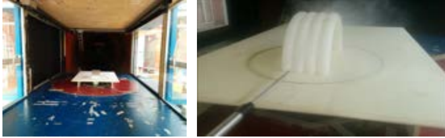
FIGURE 4. Pictures of the experimental setup to realize a uniform inlet profile.
