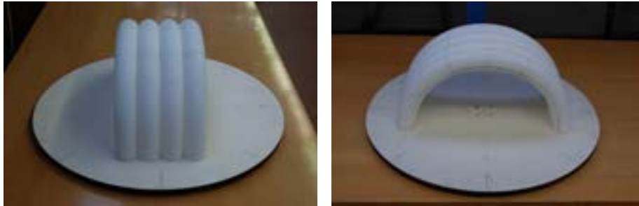
FIGURE 3. Pictures of the shelter model used for the wind tunnel tests.
