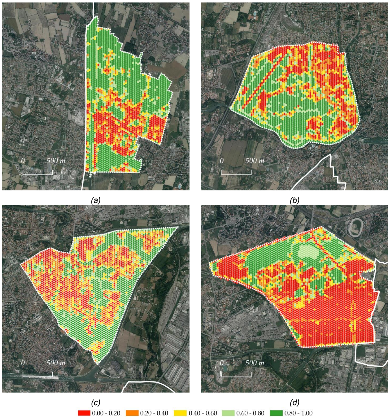
Figure 9. Hexagon tessellation of the BAF analysis in each neighborhood. (a) Brentelle neighborhood; (b) Basso Isonzo neighborhood; (c) Forcellini neighborhood; (d) San Lazzaro neighborhood. (e) Legend of hexagon tessellation
