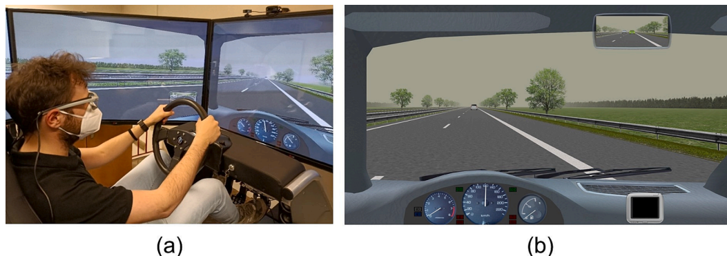
Fig. 1. Driving scenario: (a) driving simulator setup; (b) virtual environment viewed by the participant.
