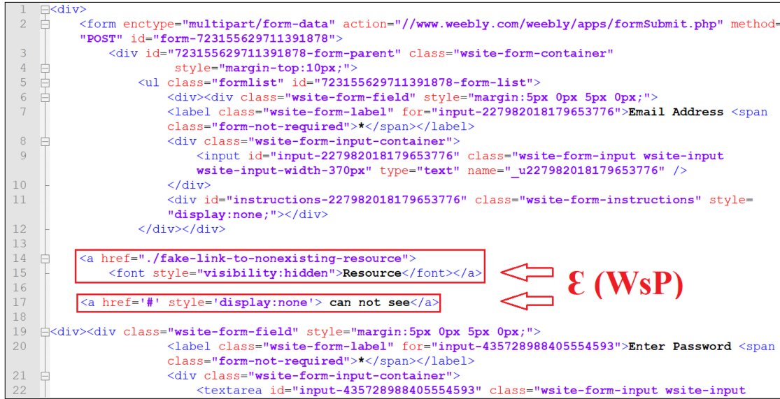
Fig. 5. A perturbation \varepsilon in the website-space (WsP). The original HTML (related to the website in Figure 4) is modified by introducing hidden link(s) . Such WsP will not be noticed by a user.
