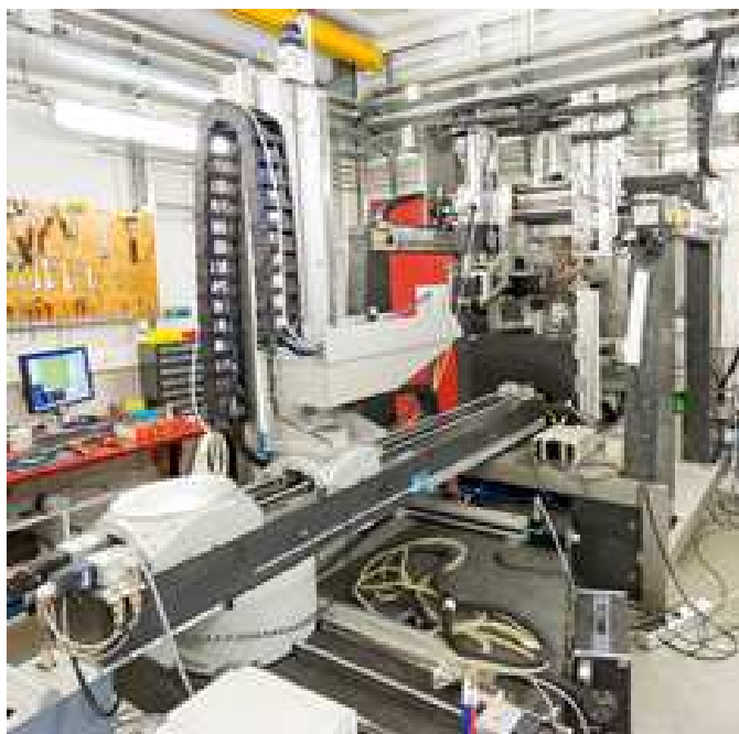
Figure 3.13: The high-resolution X-ray diffractometer in the experimental hutch of the ID11 beamline. Image taken from [33].
