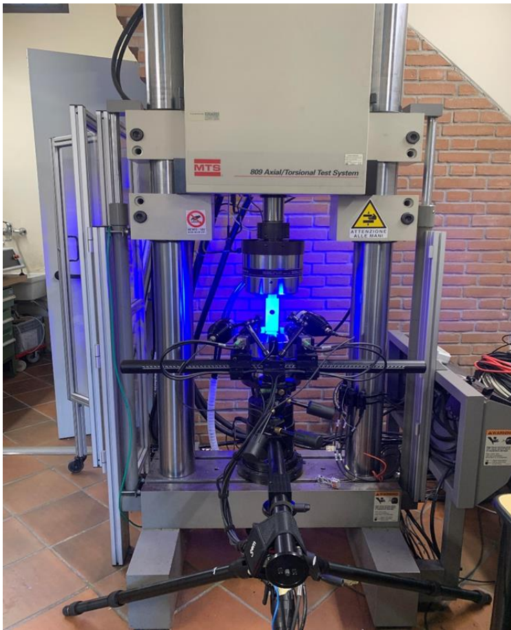
Figure V.28. Testing set-up for tensile testing and DIC measurement.
