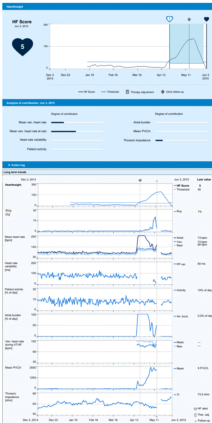
Figure 1 A reconstruction of the HeartInsight dashboard on the Biotronik Home Monitoring platform generated with data from a case included in our analysis. The dashboard consists of four segments. The first segment shows the current HF Score (5) calculated by the HeartInsight algorithm, temporal trend of HF score, programmed nominal threshold for alerts (default 45), recovery threshold (calculated as nominal threshold minus 10), and the date of the alert to worsening HF (April 22). The second segment visualizes contributions of dynamic algorithm components to the current HF Score. An Action log is available to keep track of the actions taken by the clinic in response to the alert. The last segment visualizes temporal trends of all available HF diagnostics, including percentage of CRT delivery (not included in HF score), mean heart rates, heart rate variability, patient activity, atrial arrhythmia burden, ventricular heart rate during atrial arrhythmia (not included in HF score), the number of PVC per hour, and thoracic impedance. AT, atrial tachycardia; AF, atrial fibrillation; BiV, biventricular; bpm, beats/minute; CRT, cardiac resynchronization therapy; HF, heart failure; HM, Home Monitoring; PVC, premature ventricular contractions; ven, ventricular.
