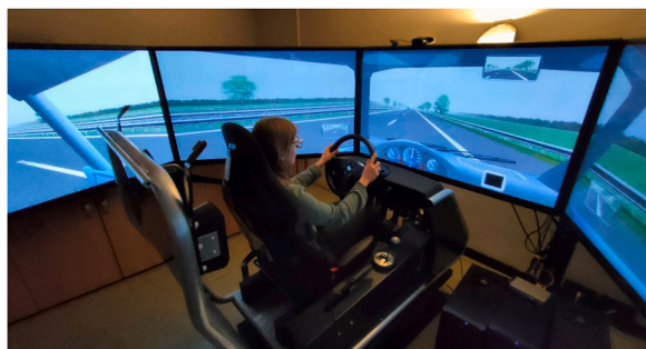
Fig. 2. Driving simulator setup and virtual environment.
