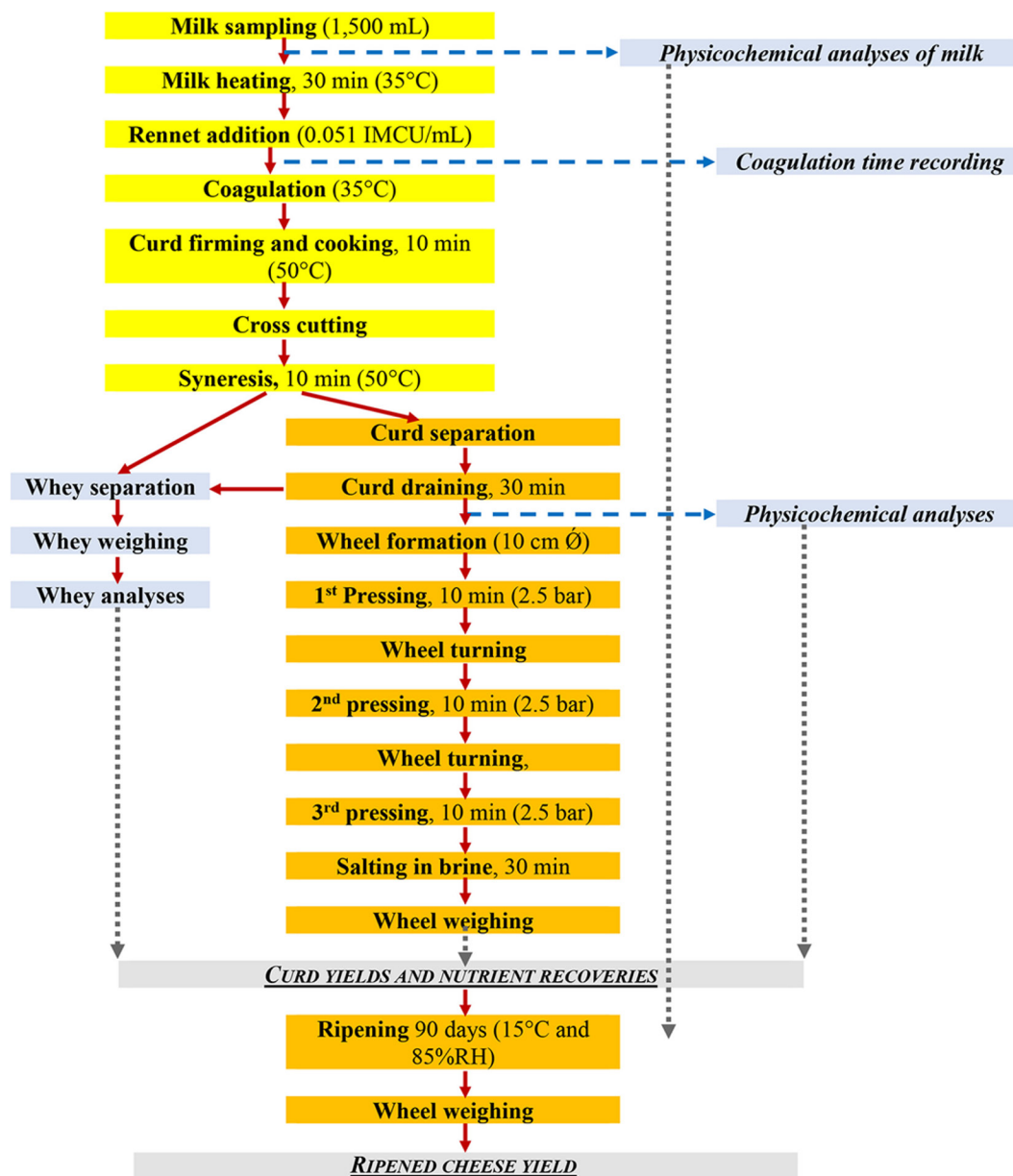
Figure 1. Workflow diagram of the model cheese-making procedure. IMCU = international milk clotting units; RH = relative humidity; Ø = diameter.
