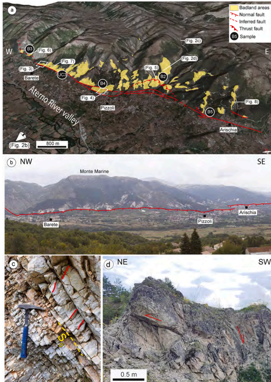
Fig. 2. Overview of the Monte Marine Fault and studied localities. (a) Perspective aerial view (Google Earth) illustrating the along-strike architecture of the MMF and the extent of the badland morphologies (in yellow) in the footwall damage zone. (b) Panoramic view of the NW segment of the MMF seen from the SW; location of photograph is shown in (a). (c) Example of the steeply dipping, well-bedded Corniola Formation host rock far from the Monte Marine Fault, affected by bed-perpendicular pressure-solution cleavage associated with the compressional phase; bedding in yellow ( S_0 ) and cleavage in red. Hammer for scale is 31.8 cm. (d) Example of the massive dolomitized Calcare Massiccio Formation affected by reverse faults with S-C fabric indicating top-to-the-NE kinematics. Steeply dipping normal faults generally overprint thrust faults. (For interpretation of the references to color in this figure legend, the reader is referred to the Web version of this article.)
