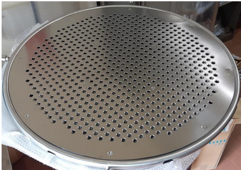
Figure 11. Picture of test #2 electrode: large double-walled shield module with staggered apertures; the apertures on the rear wall are partially visible through the apertures in the front wall.
