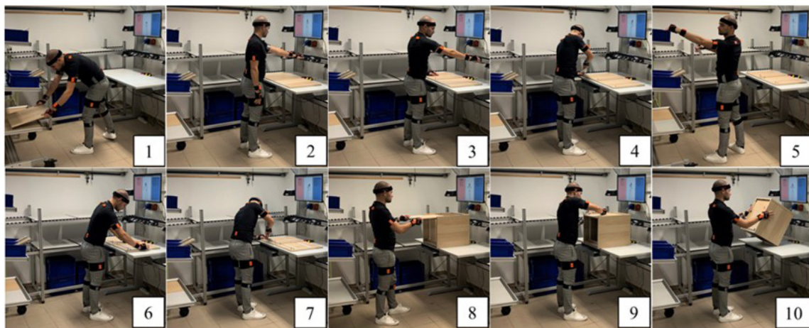
Figure 4. Ergonomic assessment of ten different postures using the digital ergonomic platform WEM (This figure/table has been reproduced with permission from Battini et al. , 2022b).
