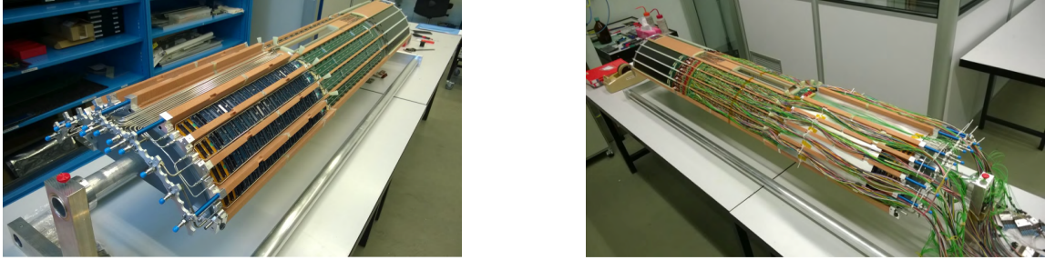
Figure 35. BPIX service half-cylinder during assembly: mechanics with power boards and cooling loops installed (left), and fully equipped BPIX service half-cylinder (right).
