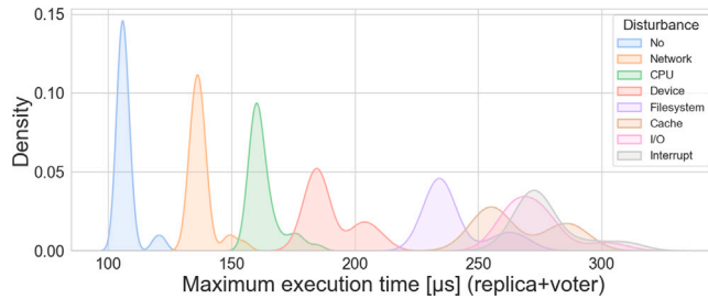
Fig. 11. Distribution of maximum execution times for the entire execution (replica + voter) by fixing host-level scheduler factor to null level, the CPU affinity factor to the One-to-One level, and varying all levels within stress factor.
