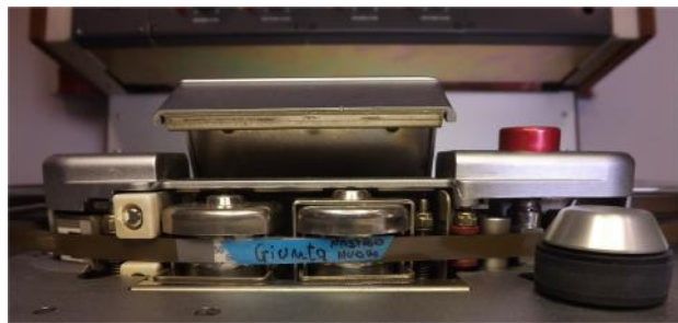
FIGURE 1. Example of markings on a tape splice.
