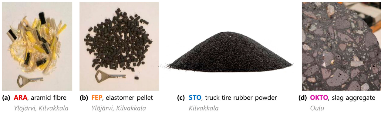
Figure 3. Examples of some materials used in the project. (a) ARA , (b) FEP , (c) STO , (d) OKTO . Notice the air bubbles inside the OKTO aggregates. Credits: Valkonen (2020), Michalina Makowska, www.veritalo.de .
