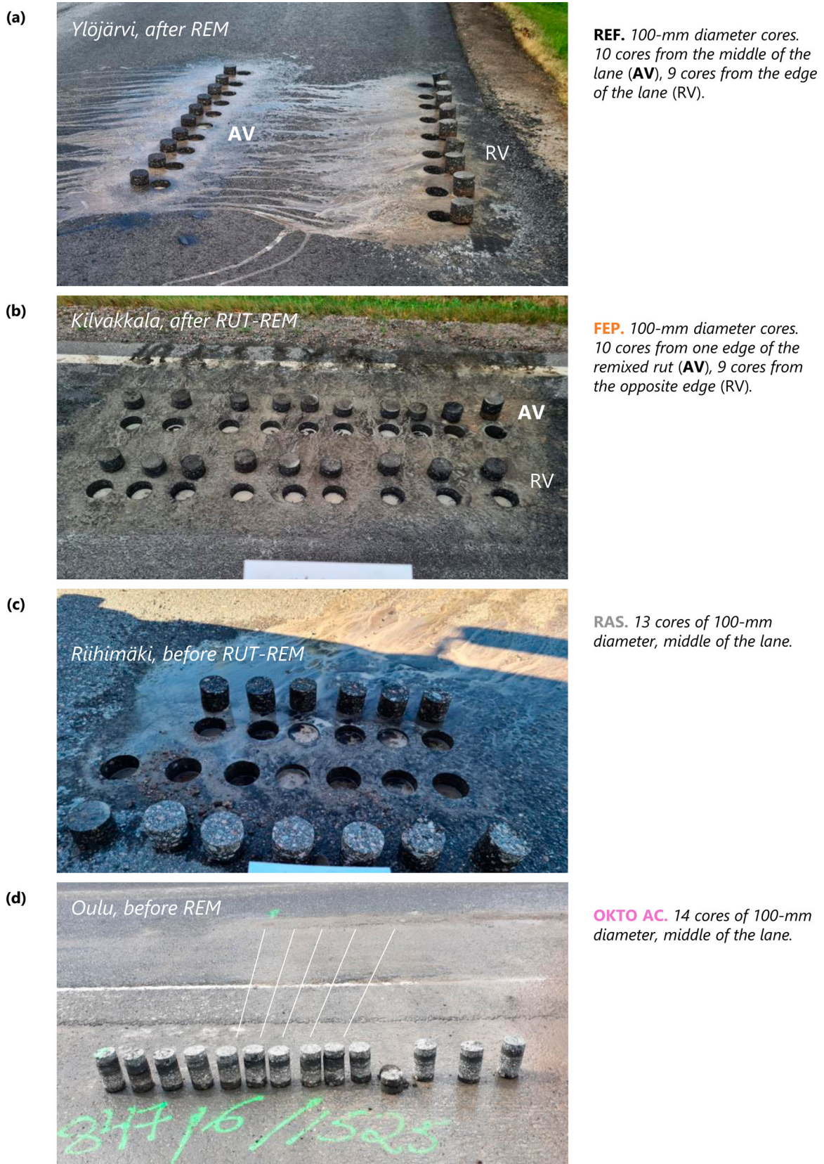
Figure 5. Selected images of the cores after extraction from the roads. (a) Ylöjärvi REM, (b) Kilvakkala RUT-REM, (c) Riihimäki, (d) Oulu.
