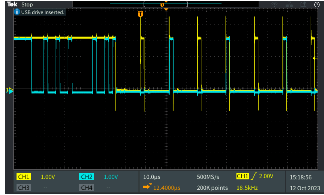
FIGURE 6.4: Start of a BOA as seen in an oscilloscope. The blue signal is the target frame (i.e., the malicious frame). The yellow signal represents the injection made by the officer. The first injection of a dominant value stops the malicious frame. Then, the following injections target error frames automatically generated by the attacker's ECU. This increases the attacker's ECU error counters, eventually reaching the bus-off state.
