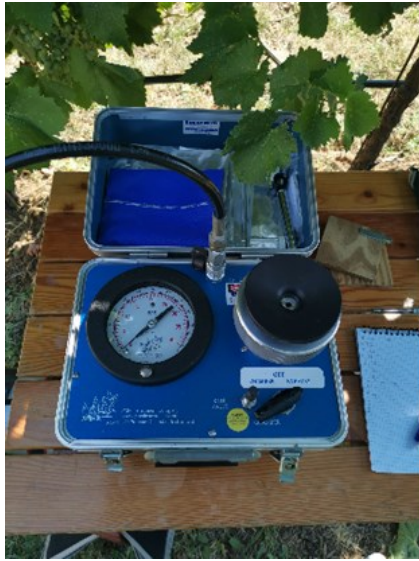
Figure 5 - Scholander pressure chamber used to measure leaf and stem water potential (model 670, PMS Instruments, Albany, USA);
