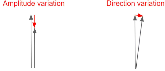
Figure 3.27: Schematic representation of the vectorial decomposition of the distortion variation.
