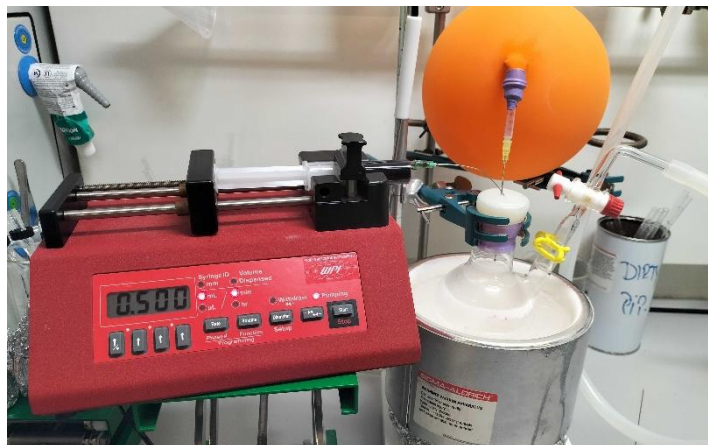
Figure 19. Reaction set-up for the synthesis of carbonyl ABBs 124 . Phenyl lithium addition is shown.
