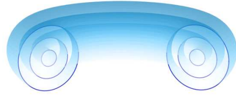
Figure 1.1: Magnetic field of a static plasma equilibrium is arranged on a set of nested toroidal magnetic surfaces.
