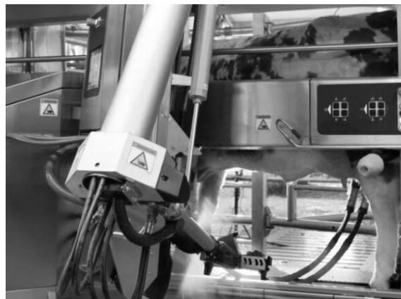
Figure 3. Robotic arm of an automatic milking system (from delaval.com).
